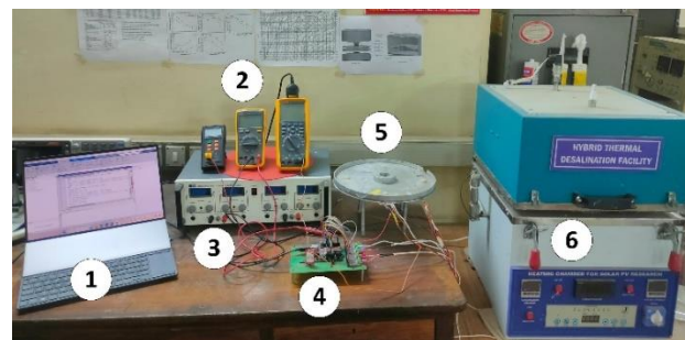
Fig 12: Experimental setup (1) logging (2) measuring instrument (3) dc power supply (4) developed temperature sensor board (5) Peltier setup (6) Desalination unit
