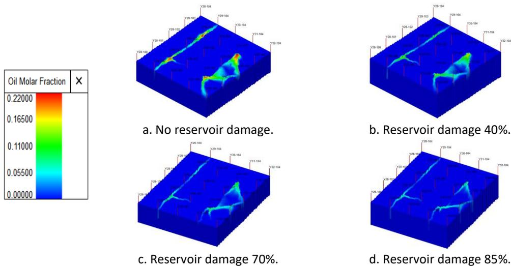
Fig. 7. CO<sub>2</sub> distribution during CO<sub>2</sub> flooding development after water flooding
