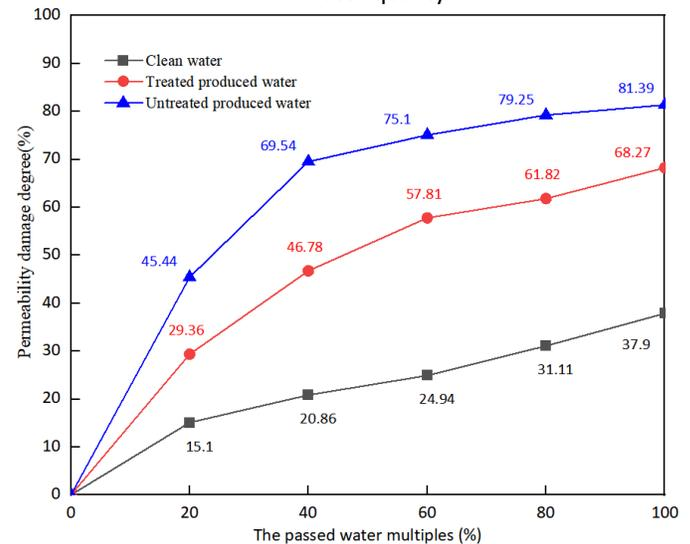
Fig. 2. Damage degree curves of core permeability with different water quality
