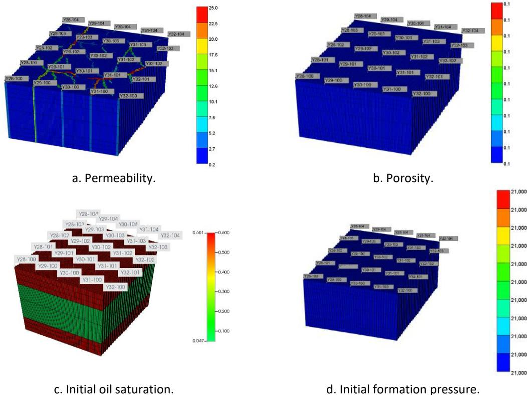
Fig. 3. Reservoir physical properties and initialization parameter fields of Y29-103—Y29-101—Y31-101—Y31-103 well group
