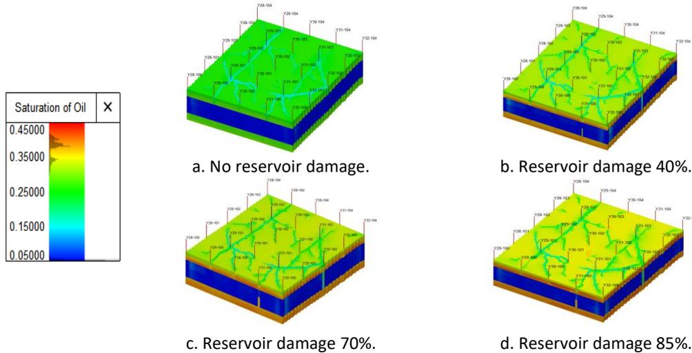
Fig. 6. Oil saturation changes during CO<sub>2</sub> flooding development after water flooding
