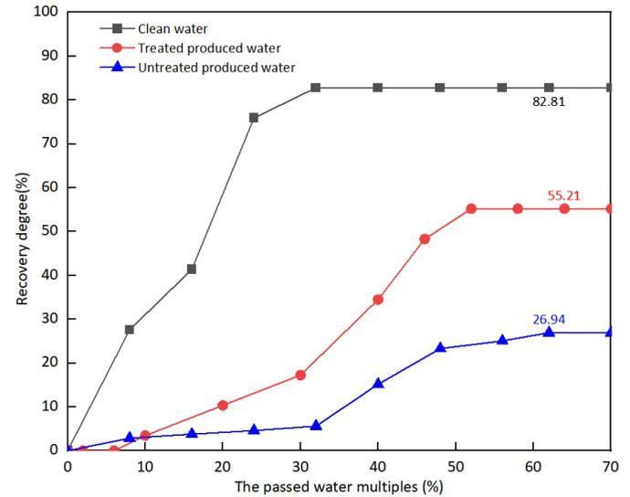
Fig. 1. Comparison of recovery factor degree with different water quality
