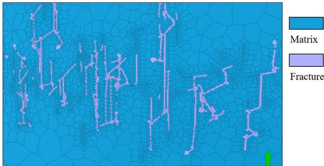
Fig. 5 The localized grid of fracture and matrix
