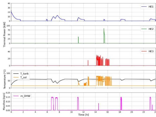
Fig. 3. 24 May: power exchanged in HE1, HE2, HE3, the tank and solar temperature, the flow rate required for the DHW
