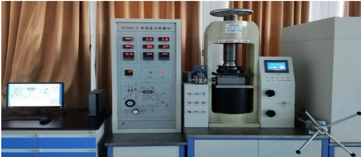
Fig. 1 FCMS-V fracture conductivity measurement system
