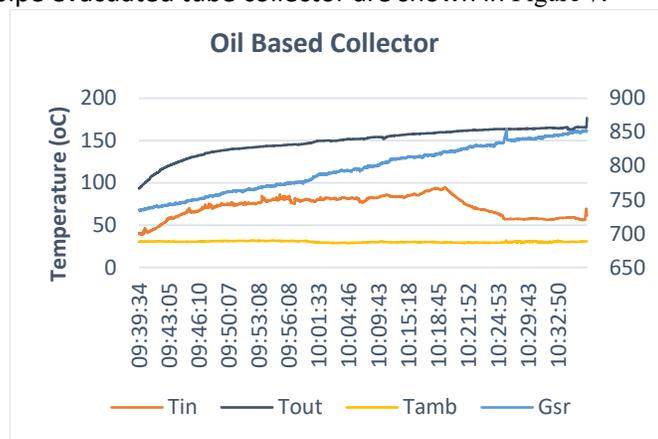
Figure 7: Heating oil with evacuated tubes. The temperatures are  $T_{in}$ : inlet to the heater,  $T_{out}$ : outlet of the heater, and  $T_{amb}$ : ambient temperature
