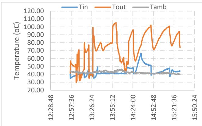
Figure 6: Heating water with evacuated tubes. The temperatures are  $T_{in}$ : inlet to the heater,  $T_{out}$ : outlet of the heater, and  $T_{amb}$ : ambient temperature.
