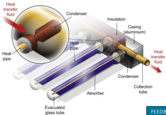
Figure 1: Evacuated tube collector components
