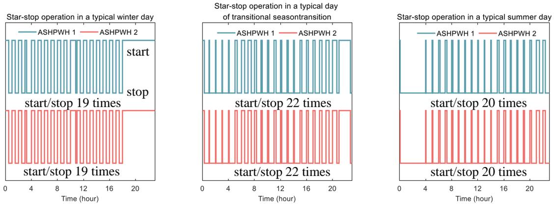
Fig. 7 Original start-stop operation of ASHPWH
