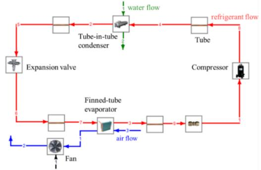
Fig. 4. Simulation model of ASHPWH in GREATLAB
