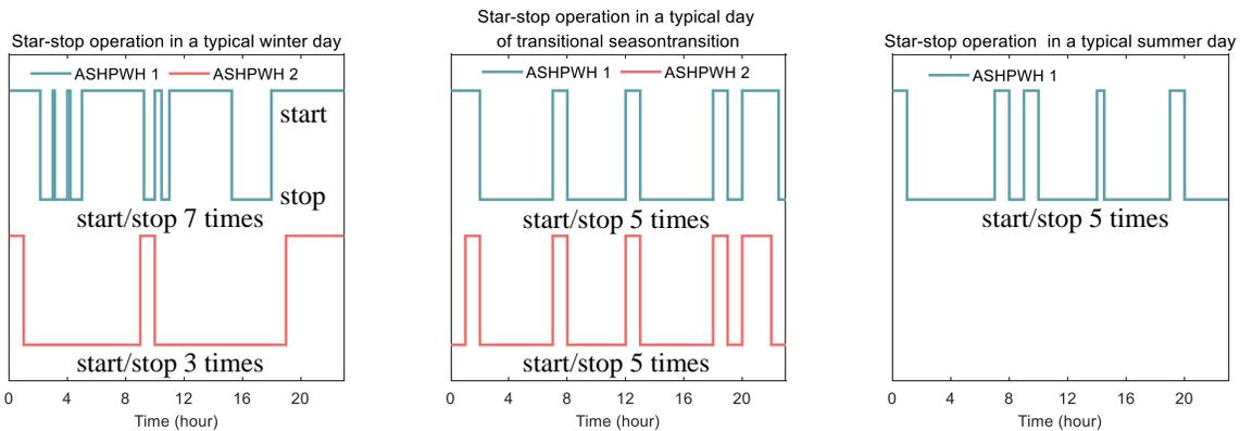
Fig. 8 Optimized start-stop operation of ASHPWH
