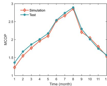
Fig. 5 Verification of MCOP of an ASHPWH
