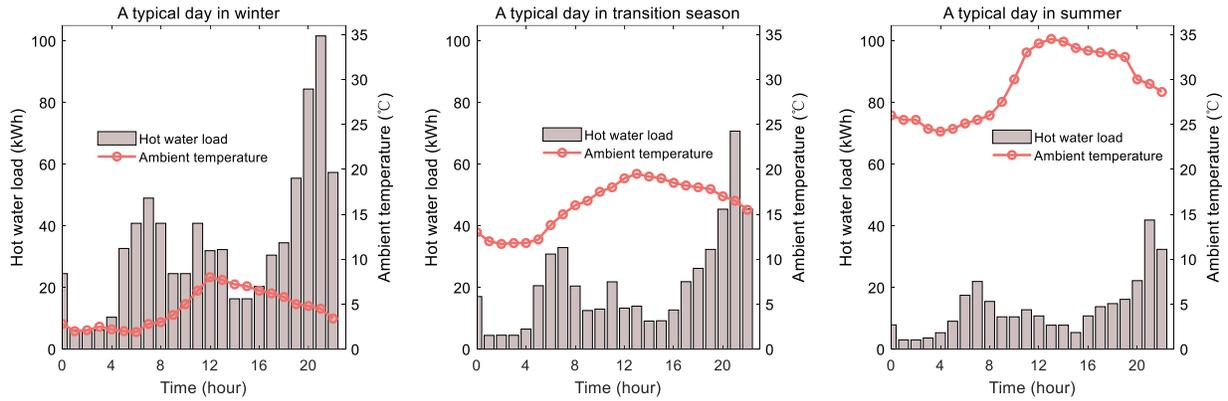
Fig. 6 Ambient temperature and hot water load on typical days
