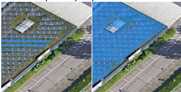
a. Points prompt b. Boxes prompt Fig. 1 Using SAM to segment PV panels
