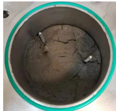
Figure2. Sediment in the Reactor
