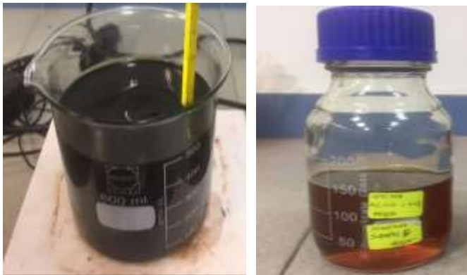
Figure 2 Left: Crude CI oil, Right: Degummed CI oil
